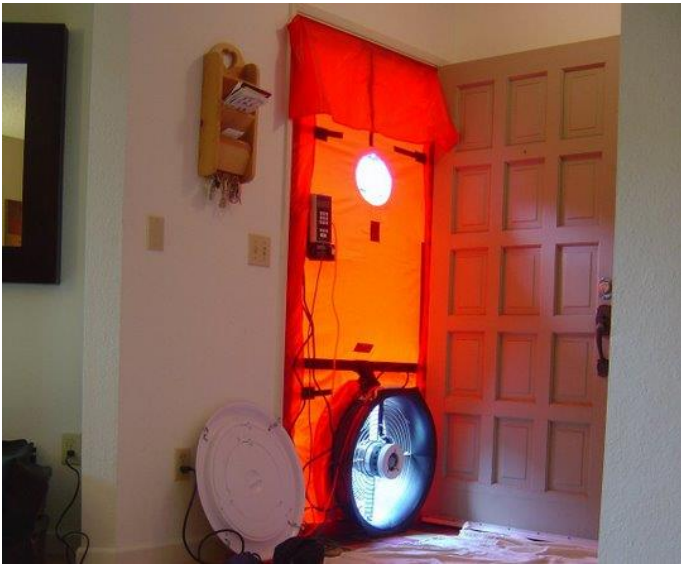
Blower door diagnostic tool mounted to exterior door
