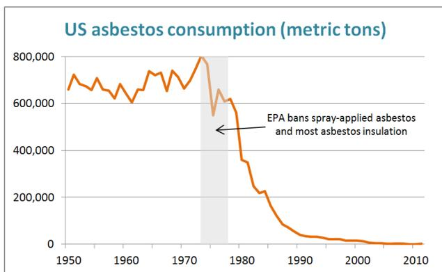
*Potentially friable applications of asbestos were banned in the 1970s. Non-friable uses such as rigid roofing materials are still legal, though not widely used. (data source: minerals.usgs.gov)*
