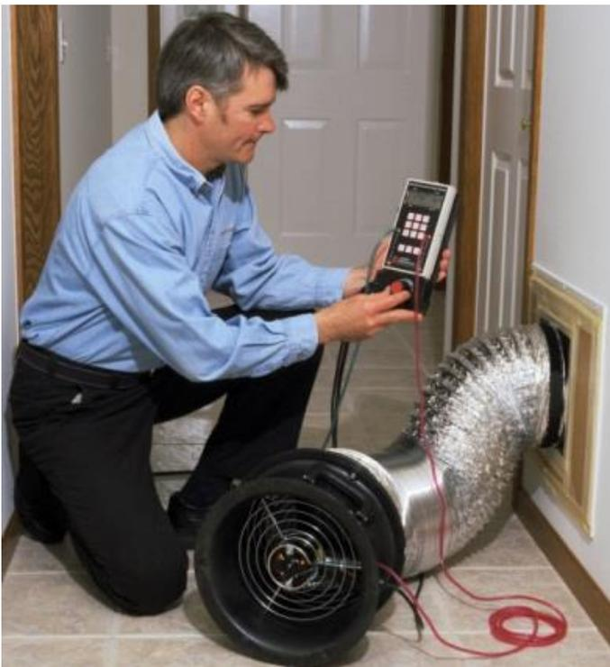
*Your contractor will perform a duct blaster test to measure the leakiness of your ducts. (source: Home Energy Pros, Lawrence Berkeley National Laboratory, 2013)*
